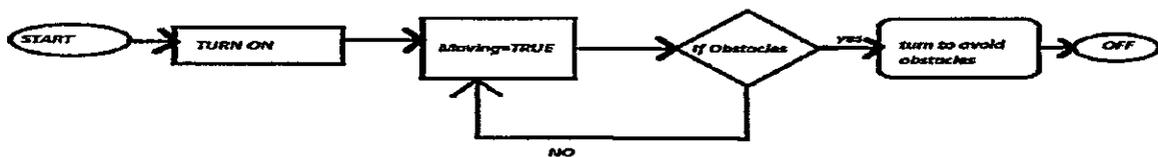
As the Robot is powered it starts moving in random pattern avoiding everything in its path. The 9V battery is facilitated with a connector for easy power ON and OFF. The battery powers the Motor Driver which is merged with Arduino Board. The power is distributed to each RO motors and ultrasonic sensor. The speed of the motors is assigned in the code and the motor can rotate in both directions as needed which comes in handy for the obstacle avoidances. when the US 015
